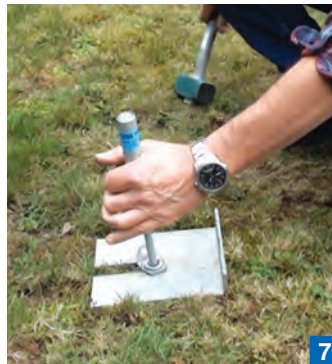
Use the sleeve to deploy the rods in the ground.
