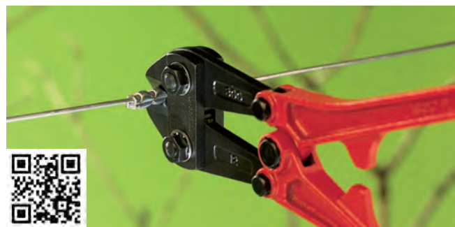
Crimping sleeve during crimping. Scan to view the video.
