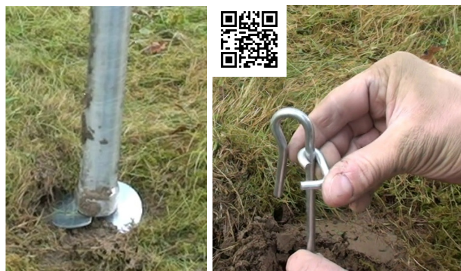
Helical anchoring disk with tubular driving tool. Scan to view the video.
